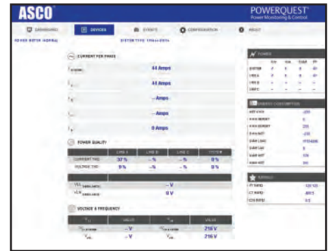
Fig. 18: Power Metering Screen
